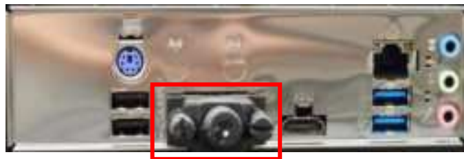
Back Panel View showing placement of MPEG “dongle”
