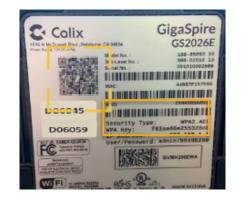
Note: The SSID (network name) of your new GigaSpire will be 'Calix GigaSpire WiFi' when the system has checked into Calix Support Cloud. The password remains the default setting; as found on the bottom of your GigaSpire (or on the sticker that came in your box) beside 'WPA Key'.
