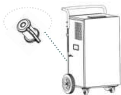
Connect a drain hose with 12 mm inner diameter to the water drainage connection.
