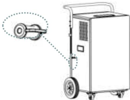
Insert a water hose with an inner diameter of 5 mm into the water drainage connection of the pump (access is possible at any angle).
