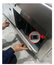
2.Unscrew the oil mist filter of the vacuum pump and fill it with oil. The oil level should not be lower than half of the oil window. The oil level should not exceed 3/4 of the visible oil window. It is strictly prohibited to start the vacuum pump without oil. (Note:two vacuum pumps)
