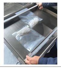
6.Press the front end of the vacuum cover by hand during operation. When operating, press the edge of the vacuum cover by hand, and the vacuum machine starts to work. After the vacuum machine starts to run, the hand leaves the machine, the ①VACUUM metre pointer will point 0.06-0.08 to achieve the vacuum purpose, and the machine will automatically complete the packaging process.
