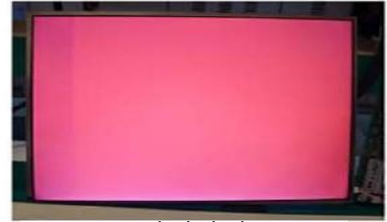
Vertical Block Source TAB IC Defect
