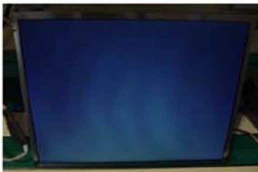
Panel Mura, Light leakage
