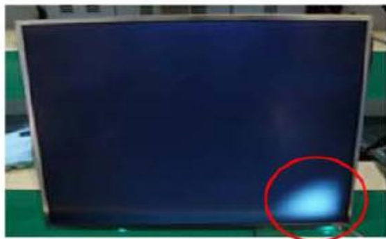
Panel Mura, Light leakage
