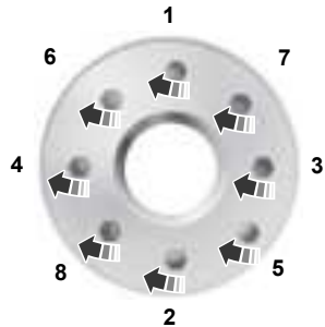
8-lug nut torque sequence.
