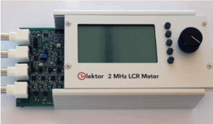
15. Partially assembled LCR-meter during the settings.
