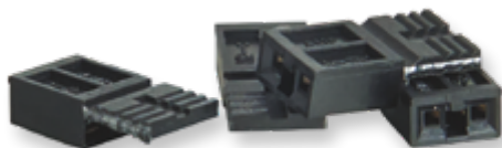
10. Four jumpers for settings during calibrations.
