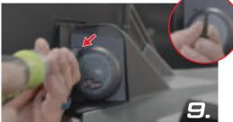
Set the tweeter and mount onto the vehicle and secure it using the included black buttonhead screw
