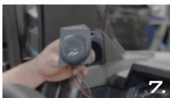
Thread the UTV Stereo onto the mount
