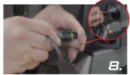
Attach the tweeter adapter to the OEM Tweeter plug
