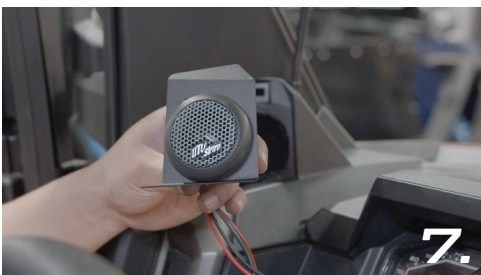
Thread the UTV Stereo onto the mount *Locking ring is not needed
