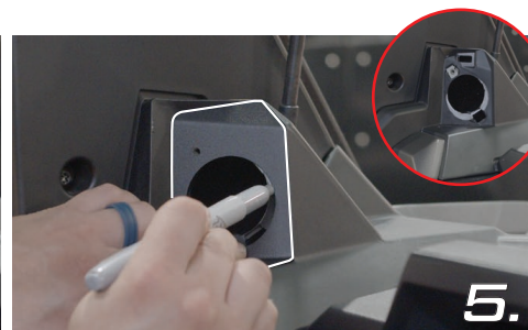
Place the tweeter mount over the OEM housing and mark the outline of the hole as shown
