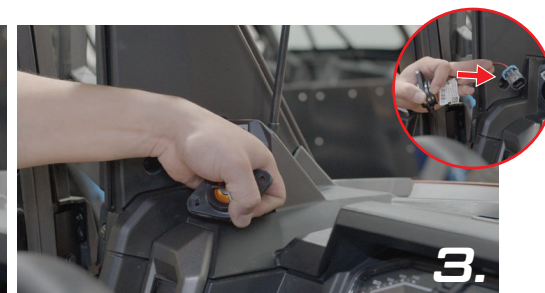
Remove the OEM tweeter *Make sure to unplug from OEM plug
