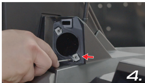
Remove the bottom metal clip
