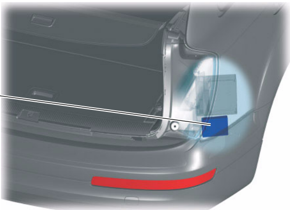
Installation location of the aerial reader unit for entry authorisation for keyless entry system J723
