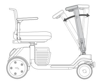
4. Tighten the tiller adjustment lever, and insert the hook at the end of the tiller adjustment lever into the inside of the lever fixing hole on the frame, and lock the lever.
