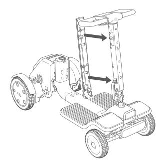
2. Install the tiller cover (front) to the front of the tiller.
