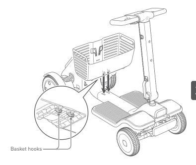
2. Take the basket hooks (2 locations) on the inner side of the basket between your fingers, and insert the ends of the basket hooks into the basket mounting holes (2 locations) on the inside of the drive base and secure in place.
