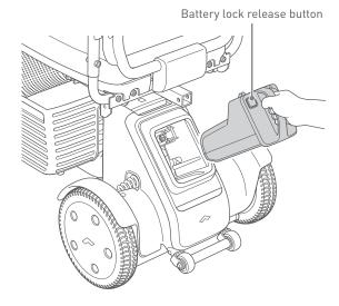
3. Grip the battery handle, and insert the battery straight until it clicks in place in the battery compartment. When it is difficult to insert the battery, push it from the front with force.
