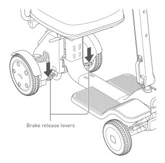
Hold the tiller handle, and move this device by pushing manually.
