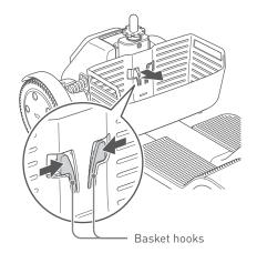
3. With the basket tilted at an angle, lift the basket straight up, and remove the basket hooks (2 locations) on the bottom rear side of the basket from the basket mounting holes (2 locations) on the base of the drive base.
