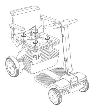
**5.** Attach the seat cushion onto the seat assembly. Secure the seat cushion and seat base in place with each of their hook and loop fasteners aligned.
