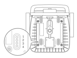
4. After determining the forward/backward position of the seat base, temporarily tighten the four locations with bolts (M6 15 mm). Then, firmly tighten to secure the seat base and seat frame in place.
