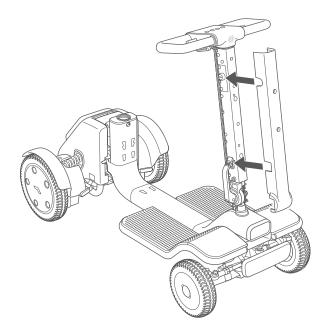
3. Secure the 4 locations on the rear with bolts (M4 12 mm).
