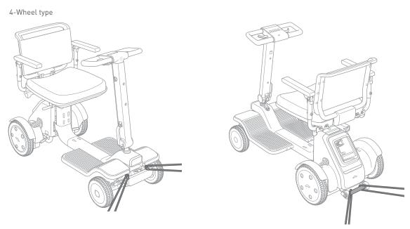
Front bumper frame and bar between anti-tip rollers (rear)
