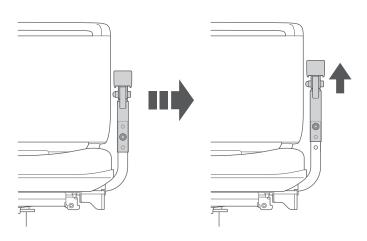
3. After determining the height of the armrest, secure with the bolt (M8 30 mm).
