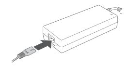
4. Remove the battery charging port cap, and connect the DC connector of the charger to the battery charging port. Connect the DC connector of the charger so that the terminal inside is aligned with the hole of the battery charging port.
