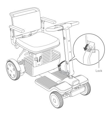
3. Adjust the tiller unit to an easy-to-use angle.
