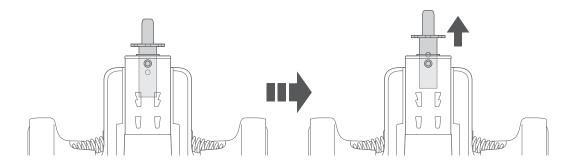
6. Tighten the seat post bolt (M10 60 mm) to secure the height of the seat post.
