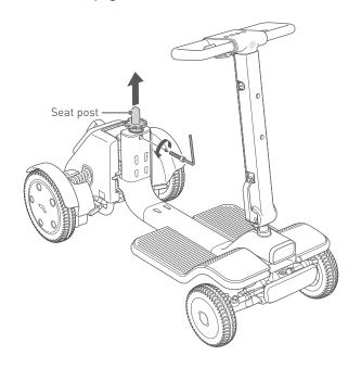
5. Change the position of the hole to align the seat post to an easy-to-use height.
