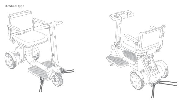
Footrest frames near anti-tip rollers (front) and bar between anti-tip rollers (rear)
