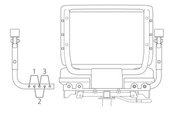
3. After determining the spacing between the armrests, secure the two bolts (M8 30 mm) in the updated positions.
