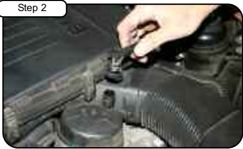
Disconnect vacuum line and pull back.
