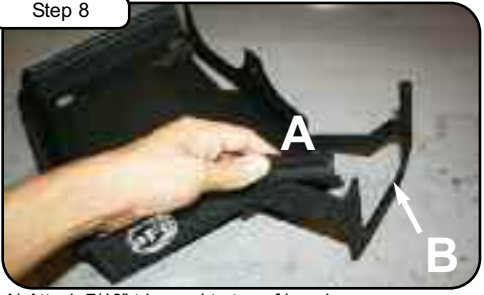
A) Attach 7/16" trim seal to top of housing. B) Attach rubber edge trim seal to ram air cut out on housing.
