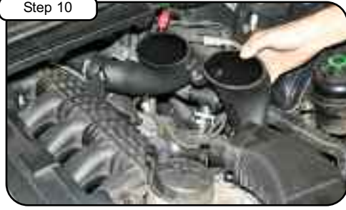
Install new tube into vehicle and pull back towards driver fender. Do not tighten clamps.
