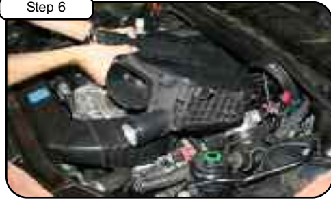
Remove complete air box from vehicle.
