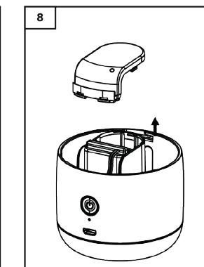
2. Remove the top cover of the product (fig. 7), and use a flat object, such as a small flat-blade screwdriver, to pry open the battery cover (fig. 8).
