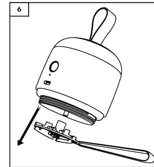
2. Install the blade by holding its plastic edge with your fingers or a pair of tweezers. Align the hole on the back of the blade with the cylinder and press the blade into position (fig. 5). Then put the bottom cover back and screw it back on (fig. 6).
