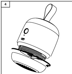
1. Remove the blade by twisting the bottom cover clockwise (fig. 3) until it is unscrewed completely. Hold the plastic edge of the blade with your fingers or a pair of tweezers, and pull it down slightly to take out the blade (fig. 4).
