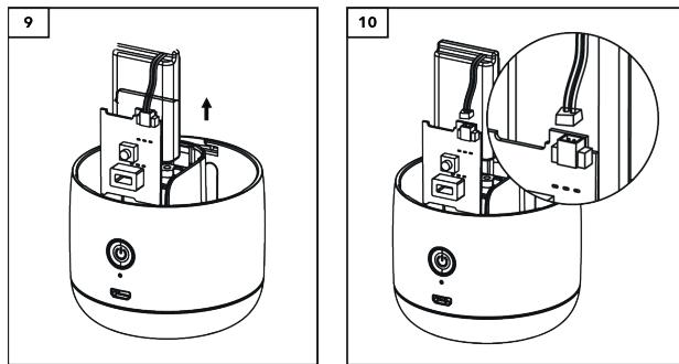
3. Remove the adhesive on the back of the battery, pull out the circuit board and the battery (fig. 9) and disconnect the battery from the circuit board (fig. 10). You can now safely remove the battery.
