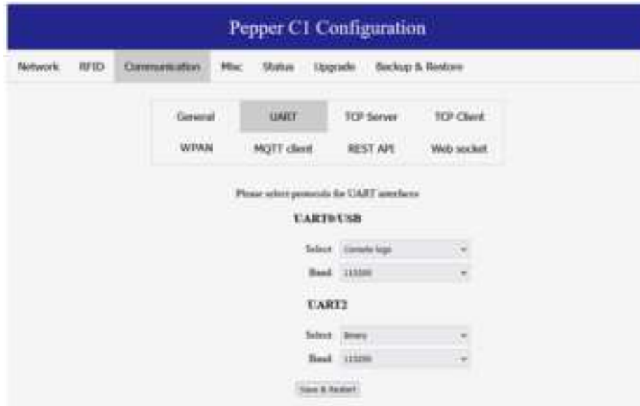
Figure 3-2. Console logs on the UART0/USB
