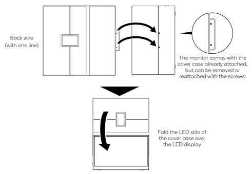
By using the cover case as a stand, the main unit can be used at an angle as shown below:
