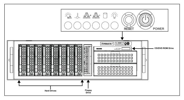
Figure 2-1. The Vertigo XG's front panel components
