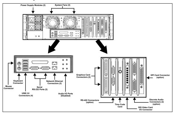
Figure 2-2. The Vertigo XG's rear panel components
