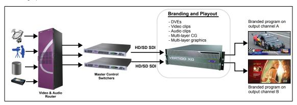
Figure 1-2. Downstream branding on two channels using the Vertigo XG
