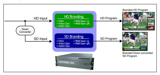
Figure 1-4. Simulcast downstream branding using the Vertigo XG
