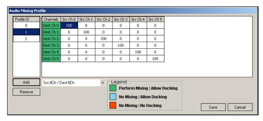
Figure 5-20. Audio Mixing Profile dialog box with a 6 x 6 matrix mixing profile
