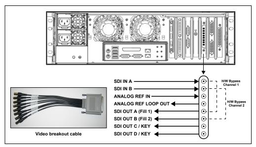
Figure 2-4. The Vertigo XG video card's input and output connections
