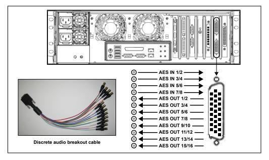
Figure 2-5. Vertigo XG's discrete audio channels
