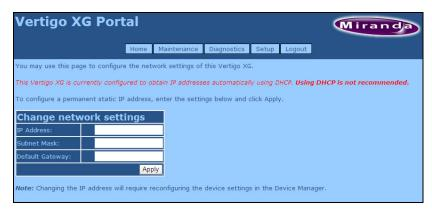
Figure 4-8. The Vertigo XG Portal's Network Setup page
