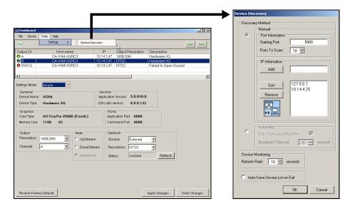
Figure 5-4. Launching the Device Discovery Tool
