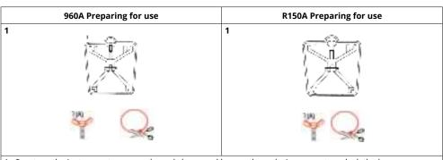
Overturn the instrument: remove the red clamp and loosen the red wing screw to unlock the lever mechanism
