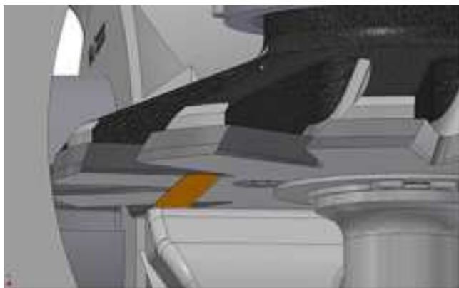
(a) Feeler Gauge Placement (Side View)
