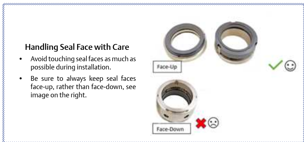
Figure 5-40. Handling Seal Face with Care
