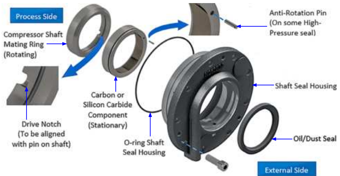
Figure 5-39. Shaft Seal Assembly
