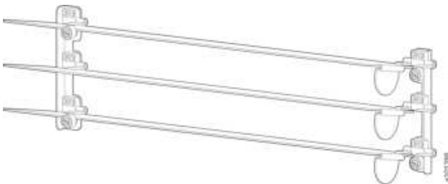
Figure 366: Air Baffle - Adjustable Louvers
