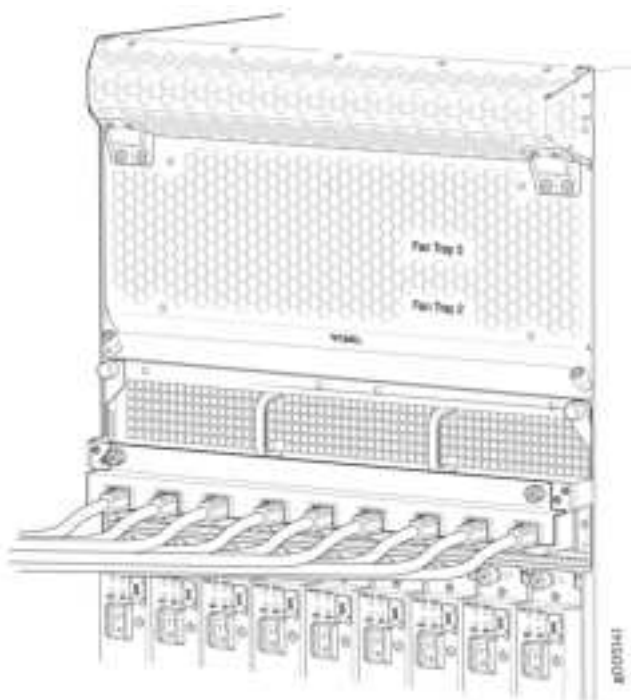
Figure 229: Proper Installation of the MX2000 Single-Phase AC Power Distribution Module in Chassis (nine-feed)
