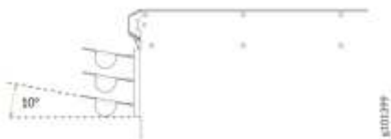
Figure 200: Air Baffle Louvers Adjusted at 10 Degrees Angle
