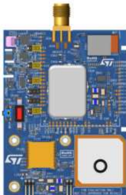
Figure 16. STEVAL-ASTRA1 jumper configuration to program STM32WL55JC
