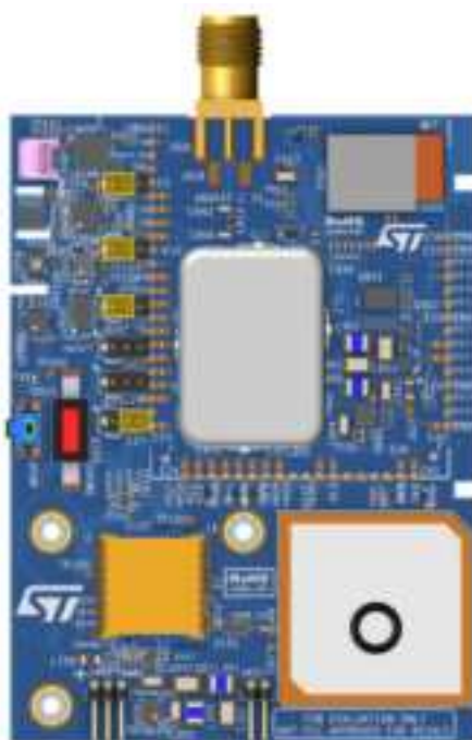
Figure 15. STEVAL-ASTRA1 jumper configuration to program STM32WB5MMG
