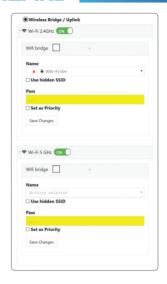
Note: The wireless radio (2.4GHz or 5GHz) selected for the Wireless Bridge will **no longer** be able to be used as an Access Point for the KE2-EM Lite. If you lose access to the KF2-FM Lite and cannot reconnect. perform a Factory Reset and select the other wireless radio for the Wireless Bridge.
