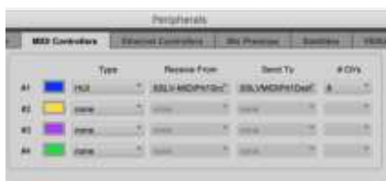
STEP 2 : Set up a HUI controller to Receive From and Send to SSL V-MIDI Port 1.
