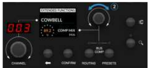
2 - Turn Secondary Encoder to move through list of functions
