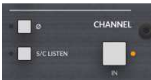
Channel Strip IN controls plug-in Bypass
