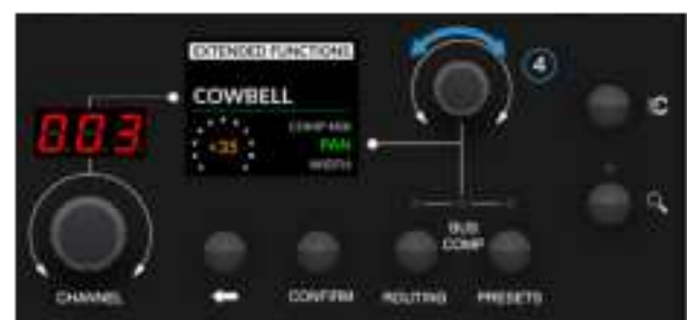
4 - Turn Secondary Encoder to adjust selected functions. Press encoder to go back to scrolling Extended Functions Parameter List
