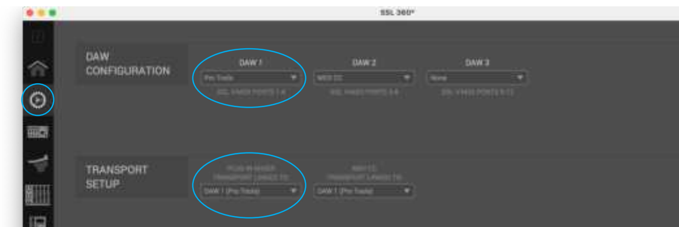
STEP 3 : On the CONTROL SETUP tab, set DAW 1 to Pro Tools in DAW CONFIGURATION and also set TRANSPORT LINKED TO as DAW 1 (Pro Tools) .
