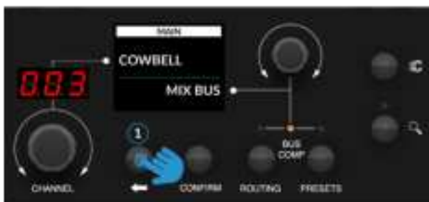
1 - Main Menu - Press Back Arrow to enter (or exit) the Extended Functions Menu Screen
