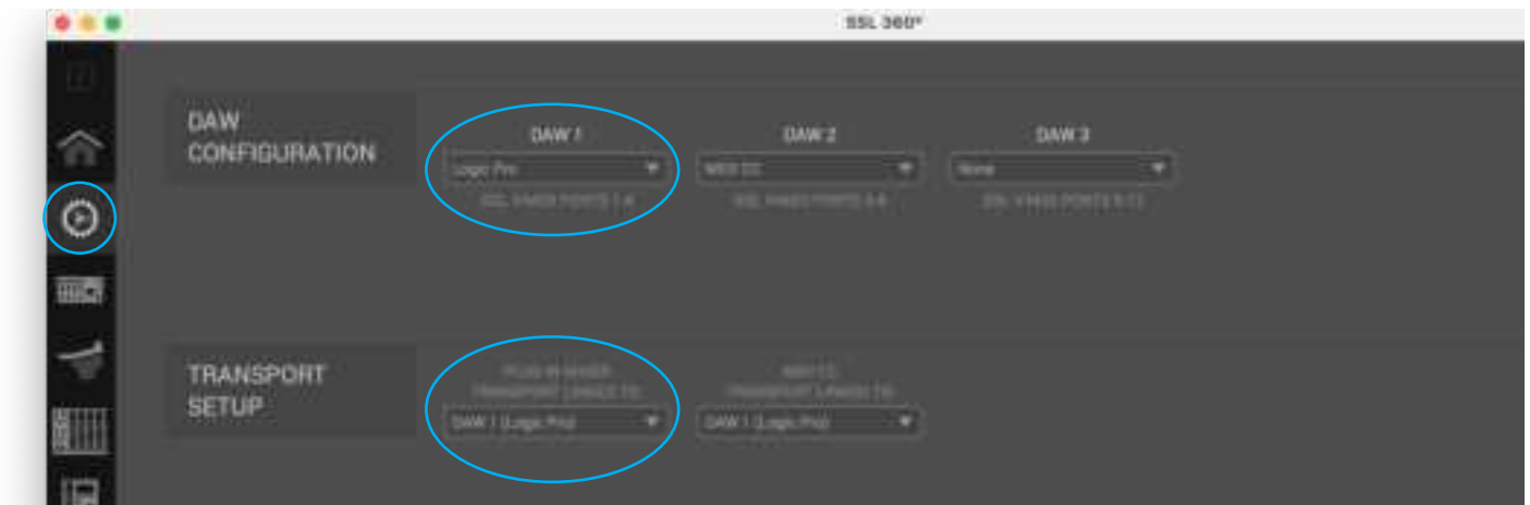
STEP 3 : On the CONTROL SETUP tab, set DAW 1 to Logic Pro in DAW CONFIGURATION and also set TRANSPORT LINKED TO as DAW 1 (Logic Pro).
