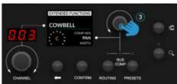
3 - Press Secondary Encoder to select function from the list to adjust
