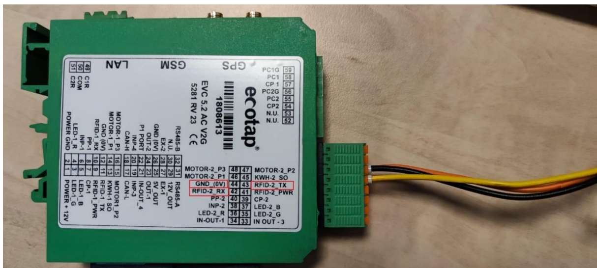
Figure 5.5 - Connecting the USB to TTL cable to the controller (EVC 5.x).
