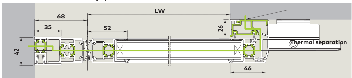
Horizontal section of lintel-mounted single-panel version
