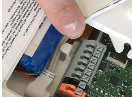
Route the wire behind the retainer clip
