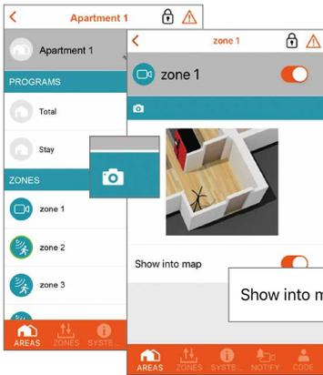
**3.5** Clicking on the individual AREAS, PROGRAMS, ZONES, OUTPUTS accesses a screen on which to assign an image (allow access to the camera).
