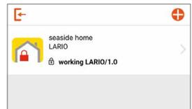
3.2 Clicking on the arrow accesses the **AREAS** section where it is possible to arm/disarm the **PROGRAMS**, to exclude/include the **ZONES** and activate/deactivate the **OUTPUTS**.
