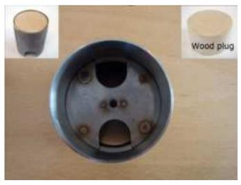
The sensor is delivered with a wood plug/cover to protect the hole when, for example, asphalt or concrete is being poured.
