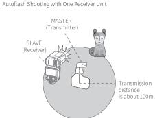
$^{\star}$  Use the supplied mini stand to position the Receiver unit.
