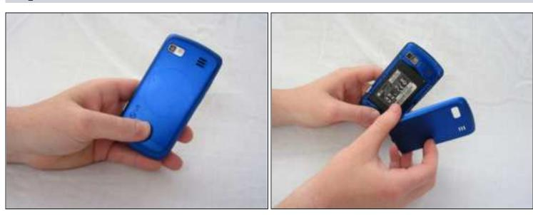
• Use your thumb to press on the small ridge at the bottom of the phone, then push upward to slide off the back casing.
