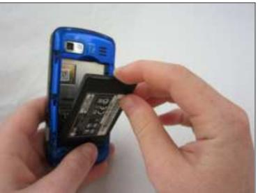
• Use your index finger to pull the top of the battery out from the top center divot. Then pull the battery towards yourself to remove it from the compartment.
