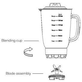
4. Place the Main Body on a flat, stable surface and then place the assembled blending cup up into the top of the Main Body and turn clockwise until it is firmly in place.
