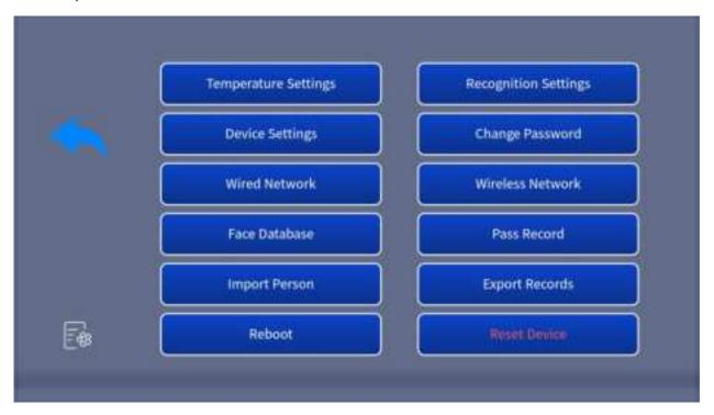
**Temperature Settings:** Click the temperature unit option to switch between Celsius and Fahrenheit; the warning value is the high temperature threshold.
