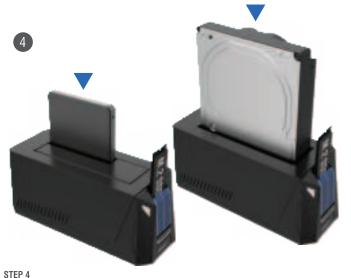
Insert the 2.5"/3.5" SSD or HDD into the top slot in the correct orientation to match the connectors; when using a 3.5" HDD the docking station must have the power adapter connected
