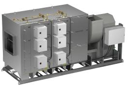
An automated wash down sequence allows for the grease buildup on the impingement filters and ESP collector plates to be removed easily with the touch of a button or an automatic daily schedule, eliminating the need to change out costly filters. Routine manual maintenance should still be conducted to ensure efficiency of the PCU.
