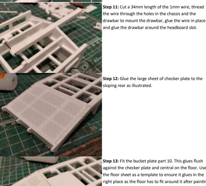
**Step 12:** Glue the large sheet of checker plate to the sloping rear as illustrated.
