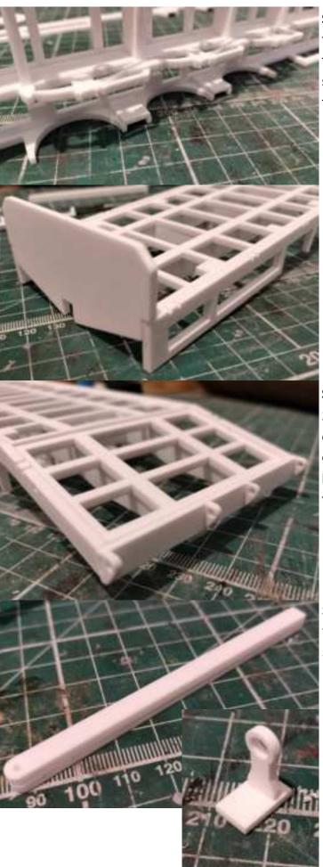
**Step 7:** Fit the side assemblies. Align the front end with the notch in the headboard, the rear should sit flush on the tops of the part 7's you glued on in step 1. This should leave the entire side approx. 1mm higher than the floor. Repeat for both sides.
