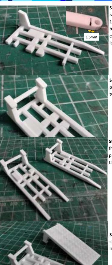
**Step 14:** To construct the ramps start by gluing the ramp frame part 12 to a ramp side part 11. Mark line 1.5mm up from the notch at the bottom of part 11. The bottom of part 12 should align with this notch. The engraved features on part 12 should point towards the leg on part 11.
