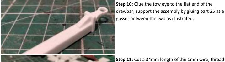
Step 10: Glue the tow eye to the flat end of the drawbar, support the assembly by gluing part 25 as a gusset between the two as illustrated.
