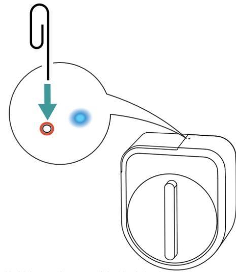
Press and hold the reset button until the blue light turns on, and continue pressing for about 2 seconds until the light turns off to complete the reset.
