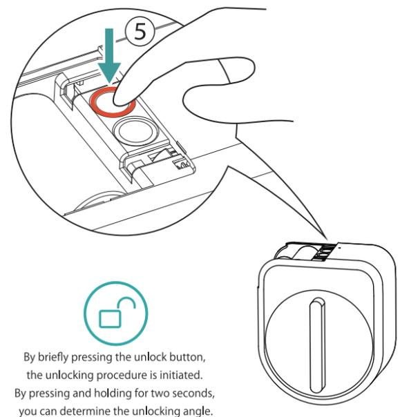
By briefly pressing the unlock button, the unlocking procedure is initiated.
