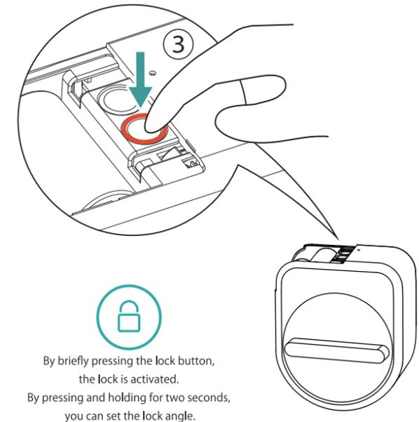
By briefly pressing the lock button, the lock is activated.
