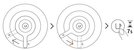
Lock the machine head by turning the lever left until the lock symbol and then unlock the lever by turning right to the unlock position. Press and hold the button again for approximately 7 seconds or until the light turns off. The button will start blinking orange rapidly.
