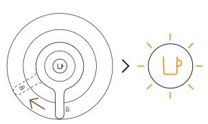
7 To enter the descaling mode, lock the machine by turning the lever left towards the lock position. The light should still be blinking orange quickly. This is an indication that you have entered descaling mode.
