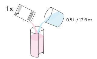
2 Fill the water tank with 0.5 L / 17 fl oz of water and add 1 unit of **Nespresso** descaling liquid.
