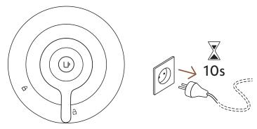
1 With the machine closed and the lever in **unlocked** position, unplug the machine for at least 10 seconds.
