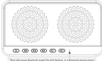
\*Blue light means Bluetooth mode(The light flashing is in Bluetooth pairing status)
