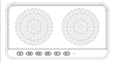
M-----Short press will input function key, switch among AUX/FM/Bluetooth mode; Long press will power switch.
