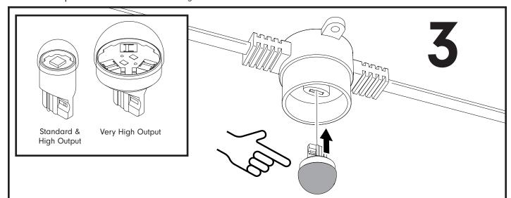
**NOTE:** If an LED does not light up after powering on the Litesphere 2.0 strand, remove unlit LED, flip 180 degrees, and re-insert into socket.
