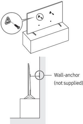
1. Using the appropriate screws, firmly fasten a set of brackets to the wall. Confirm that the screws are firmly attached to the wall.
