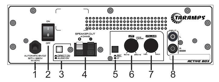
1 - **Power Cable**: Connect the cacle to the electricity network. This product operats with a power supply between 90 and 240 VAC.
