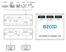
Note: When you have 4K HDMI source device, but 1080P HDMI display device, please connect 1080P display to HDMI OUT2.
