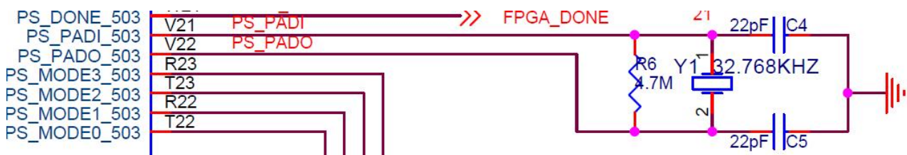
Figure 2-6-2: Passive Crystal Oscillator for RTC
