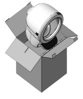
c. Slide the corner (1) and top inserts (2) into place with the power supply in the top pocket (3). Write your name and RMA number prominently on the outside of the box and on an interior box flap prior to sealing the box with tape.
