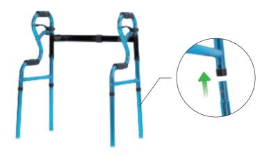
**Step 4:** Install the Rear Leg with Rubber (Part# D) and Front Leg with Wheel (Part# E) as shown.
