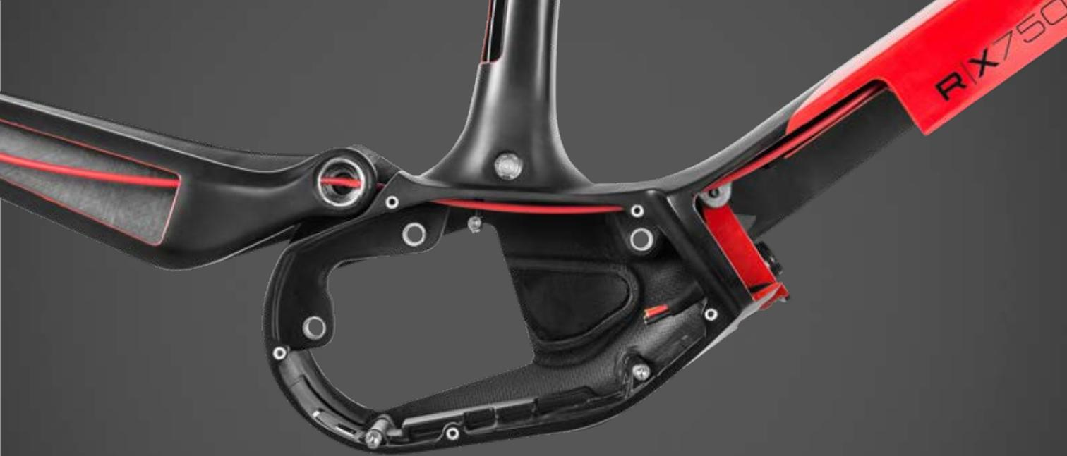
FULLY INTEGRATED CABLE ROUTING R.750
