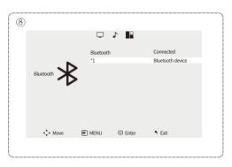
Note: The projector can only connect to INPUT devices via Bluetooth connection. Therefore, it cannot connect to mobile phones via Bluetooth to mirror your screen.
