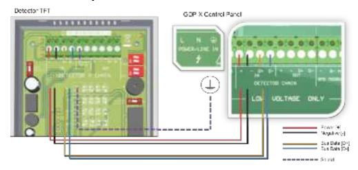
[SHEILD WIRE] detector terminals should be used for earthing/grounding and shield wires connected to any Earth/Ground terminal on the control panel. Twist the shield wire to avoid stray shield wires,
