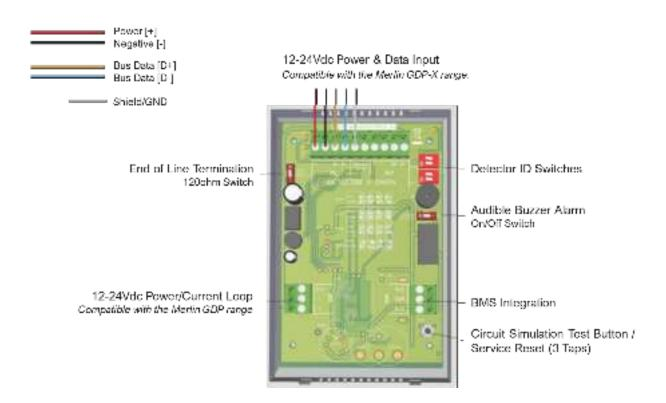
Note: Terminal blocks are plug/socket type and may be removed to ease wiring.
