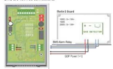
A relay will change state when in alarm or when gas is detected.
