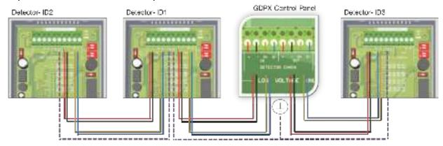
Reversing the [D+] and [D-] connections of any device can lead to the whole system to stop working owing to reverse polarity found on the terminals. In order to avoid this problem, it is recommended that the cable of same colour should be used to connect all [D+] terminals together and similarly cable of same colour to be used to connect all [D-] terminals together.
