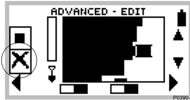
Figure 6.11 Rejecting framed target area
