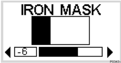
Figure 5.5 Adjusting the Iron Mask
