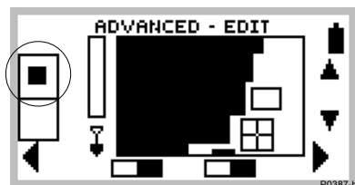
Figure 6.10 Edit screen with target crosshair and medium target frame
