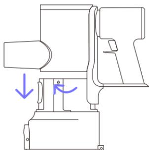
Place the arrow on the dust cup corresponding to the dust cup body unlock mark then turn clockwise to lock.
