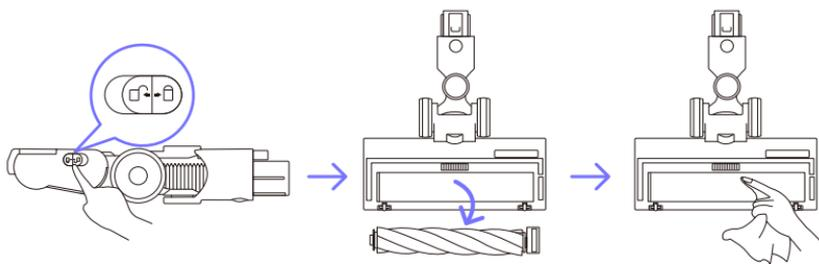
Remove the debris wrapped around the roller with Powerffy Hair Cleaning Tool, then flush with water.
