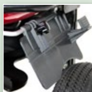
Side Baffle For directional control of spread
